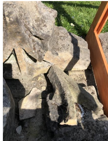
Examples of stone features having experienced material loss (left), surface flaking/chipping (middle) and stone splitting (right). Images taken by author with kind permission from Burwell Museum & Windmill .
